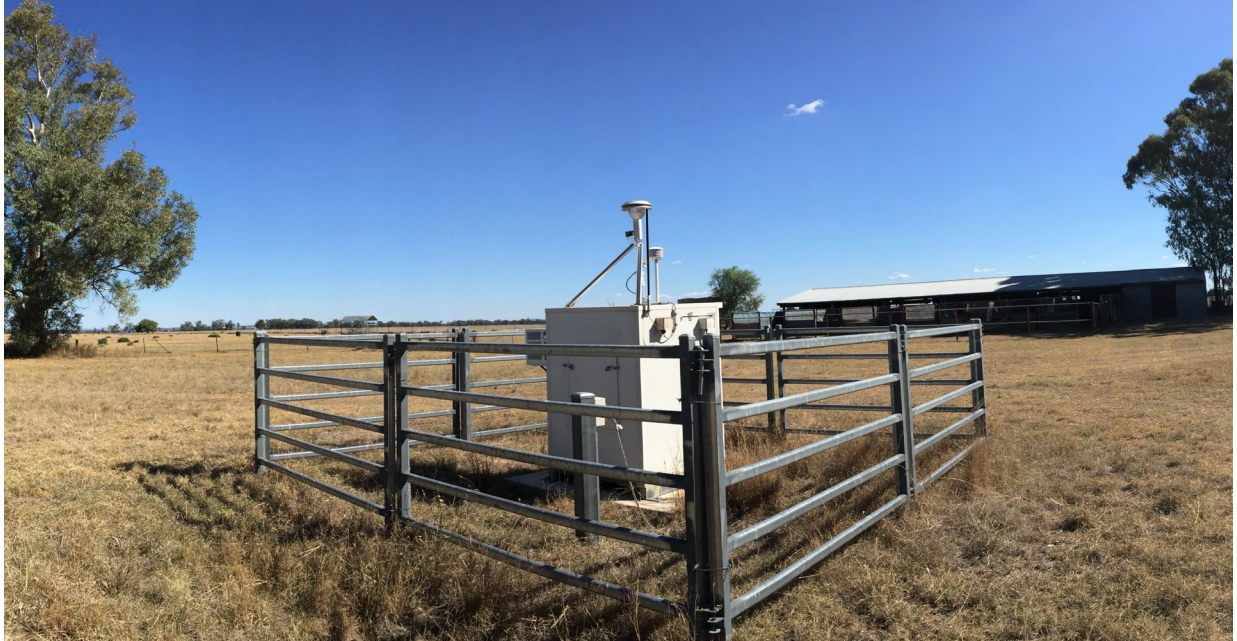
Figure 1: TEOM installed at Flixton property
