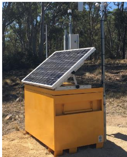
Figure 2: Portable and real-time dust monitor installed at TCM in November 2018
